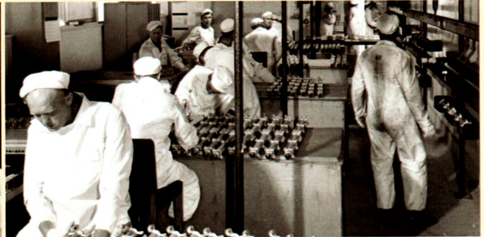
Reactor Two Fuel Preparation area showing Fuel Element inspection benches and an overhead conveyor to the reactor. September 1965.
