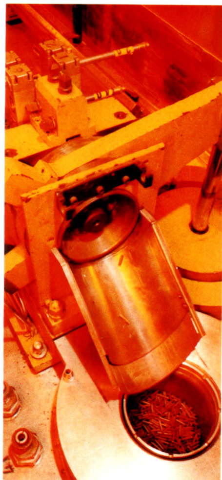
Right: The cropped pieces of fuel pins are poured into a basket before being removed to the dissolver.
