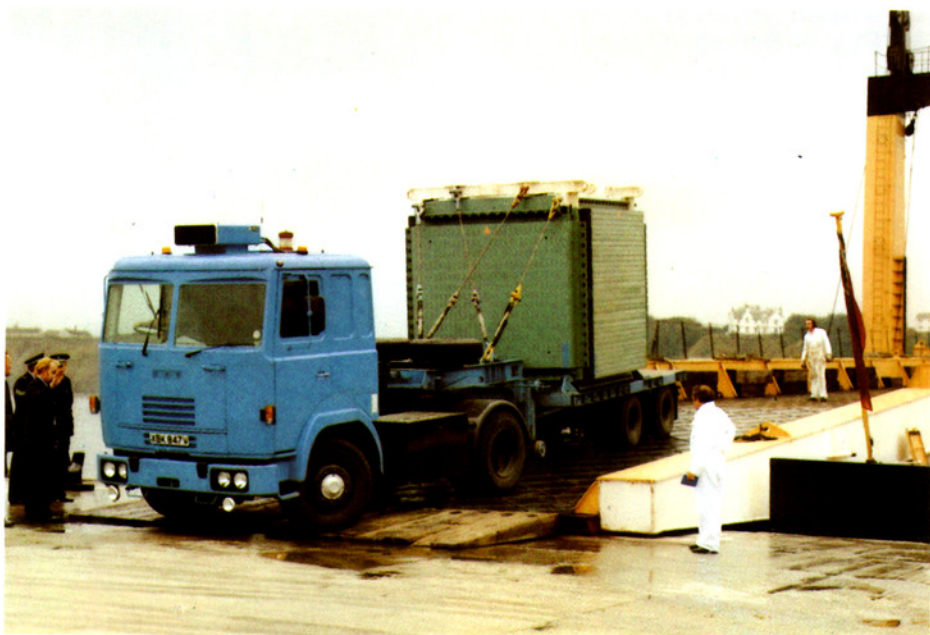
Vehicle, loaded with shielded flask used for plutonium nitrate, reversing onto vessel prior to shipment by sea to British Nuclear Fuels Ltd, Sellafield, Cumbria.
