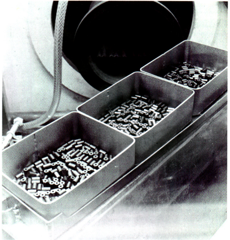
Right: Trays of PFR plutonium/uranium pellets manufactured from reprocessed fuel removed from sinter furnace.
