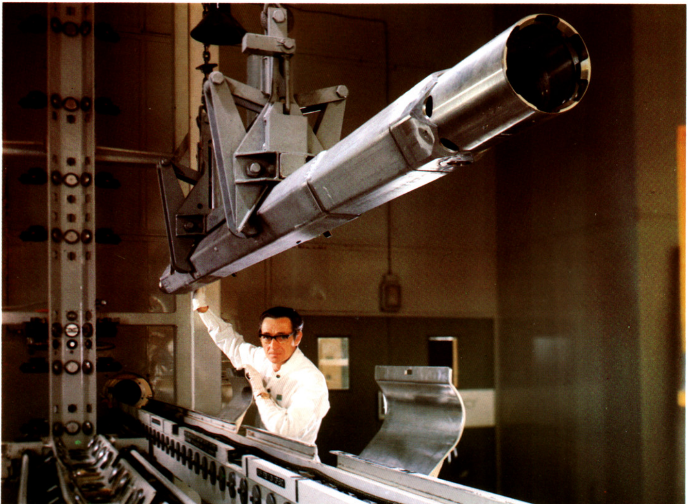
Below: A new PFR fuel assembly at Sellafield.
