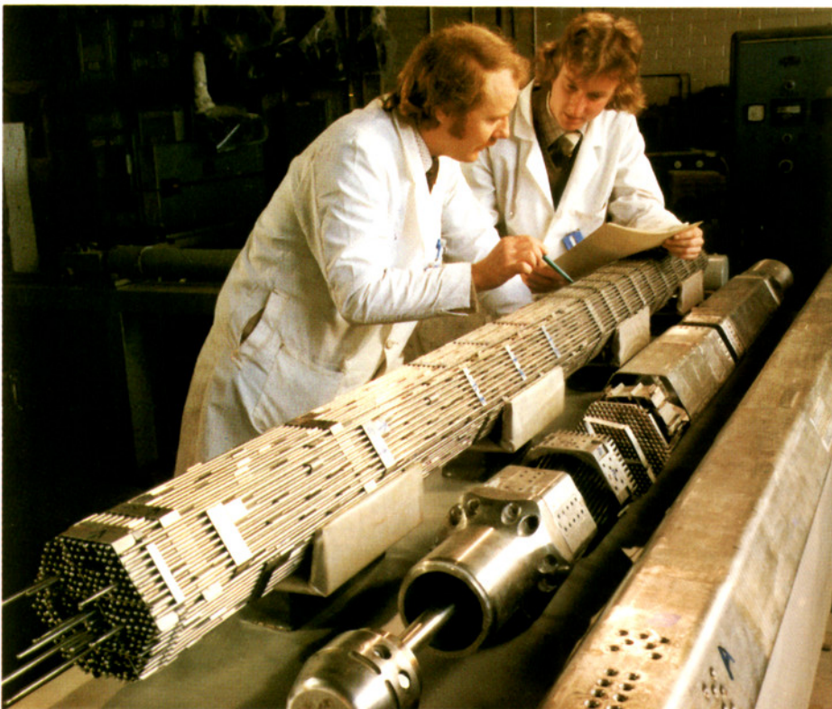
PFR fuel assembly, before irradiation, showing main component parts.
