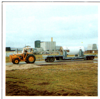
Irradiated fuel being transferred from PFR to the Reprocessing Plant in a shielded transit flask.
