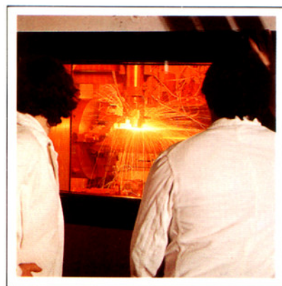
The end of a PFR hexagonal-shaped fuel assembly's outer wrapper is removed by laser cut, exposing the fuel pins.
