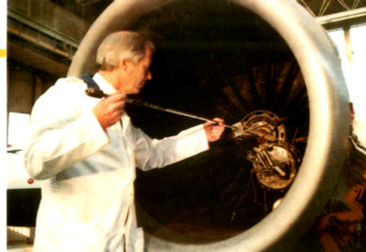
Routine inspection of a jet engine using gamma radiation
