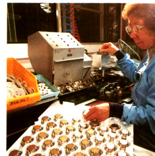
Ion chambers being assembled for use in smoke detectors
