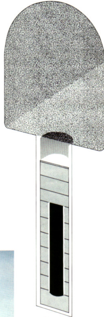
◁ Schematic diagram of a canister in its deposition hole, surrounded by blocks of highly compacted bentonite clay. The tunnel has been backfilled with a mixture of sand and bentonite.
