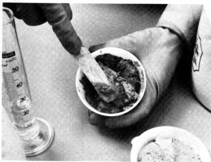
Laboratory preparation of simulated highly active waste for vitrification, at the Windscale works, in Cumbria, of British Nuclear Fuels Ltd
